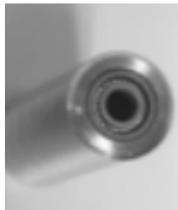
Fig. 4. New seal in replacement tool.
